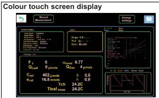
A large, colour, touch screen display makes the iFL both interactive and simple to use. Set up is easy whether loading or editing an existing protocol, or building a new protocol. Real time data, calculations and graphs are clearly presented on screen. Sub screens can be blown up to full screen size for even easier viewing.
